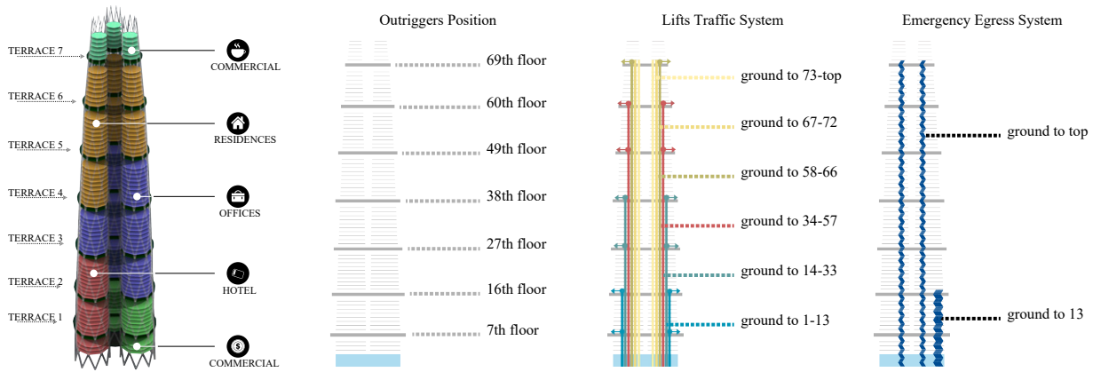
Figure 19: Architectural and functional design: functions allocation and vertical circulation.
