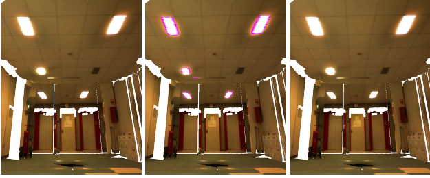
Figure 3: After the projection of the HDR data to the point cloud (left image), some points can miss HDR values or receive invalid HDR color (magenta points in the center image) stemming from low PatchMatch confidence. The image on the right shows the final result, after the gradient-domain reconstruction.
