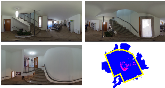
Fig. 14 Failure case. We show a scene with open ceiling, stairs and a curved wall where our method failed to recover the structure. We show some of the original captured images, the resulting (wrong) transform in the 2D plane and the expected real shape (yellow).
