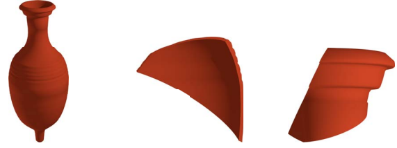
(a) A reconstructed amphora model without handles. This model has 61 vertical rings and 142 profile points. (b) Sherd with a vertical fracture. The inner and outer profiles are on the left and right of the fracture, resp. (c) Sherd without a vertical fracture. Its right side is aligned to outline the outer profile.
