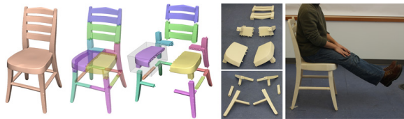
Figure 9: The Chopper approach, designed to overcome the working space limitations of current 3D printing technologies.
