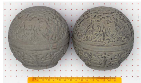
Figure 10: The colour-enhancing technique: a comparison between the plain replica (left) and the version with colour enhancement (right).
