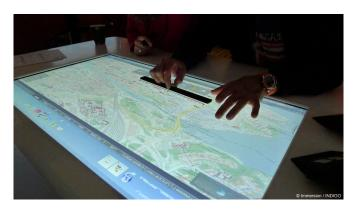
Fig. 4. **INDIGO Tangible Ruler.** Users are able to mesure digital maps with a tangible ruler. The digital scale around the objects automatically adapts to the maps scale.
