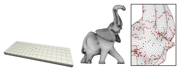
Figure 3: Left: An otherwise semi-regular quad meshing of a bar includes two irregular vertices (in red) in order to change tessellation density from six quads (left end of the bar) to five (right end of the bar). Right: A quad-mesh with adaptive density. Adaptivity (i.e., quad size adapting to local shape complexity) is obtained at the expense of introducing many singular vertices (in red).
