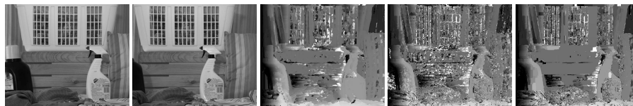
(a) Reference Frame (b) Match Frame (c) DM from WTA (d) DM from SA (e) DM from GC
