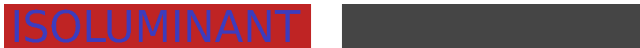
Fig. 1: Isoluminant changes are not preserved with traditional color to grayscale conversion. Converting a blueish text whose luminance matches that of the red background to grayscale can result in a featureless image.
