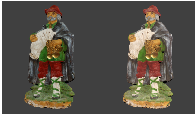
Fig. 12. An example of color correction result, visualized with no illumination (only color values assigned to vertices); color correction is OFF in the left-most image and ON in the right-most one.
