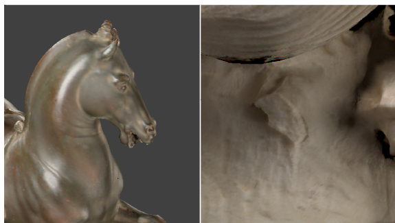
Fig. 9. Details of two colored models produced with (no flash images), visualized without illumination and shading (only color values assigned to vertices): multiple highlights show up on the digital models (left); the presence of shadows and different illumination between photos generates a non completely continuous color (right).
