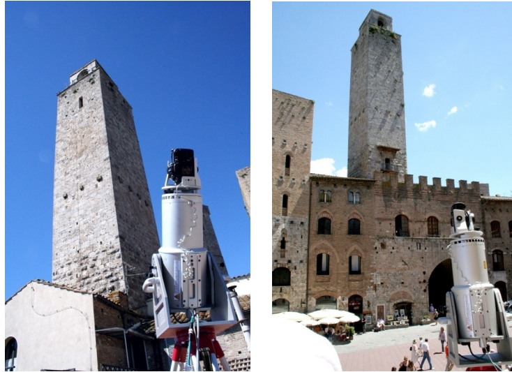
Figure 1. Acquisition of the tower's geometry by means of a TOF laser scanner.
