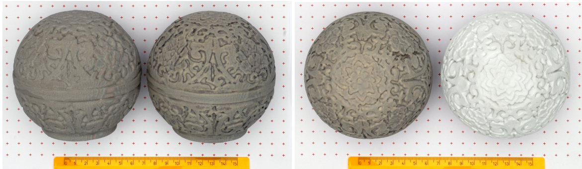
Figure 6: The color-enhancing technique compared with a white painted version of the "Red Circular Box" model. In the left pair the comparison between the plain version and the version with the color enhancement. In the right pair the color enhanced version compared with a model that have been painted with a very opaque diffuse white paint that should remove most of the SSS optical effects.
